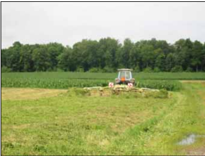
The picture to the right is an example of the OxBo/Miller Pro Merger. You can see its full width pickup head. It will pick up a 30 ft. swath of hay.
