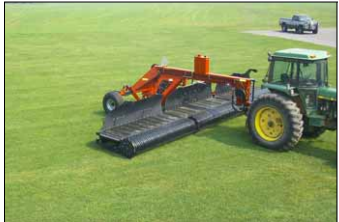
The picture to the right is an example of the OxBo/Miller Pro Merger. You can see its full width pickup head. It will pick up a 30 ft. swath of hay.
